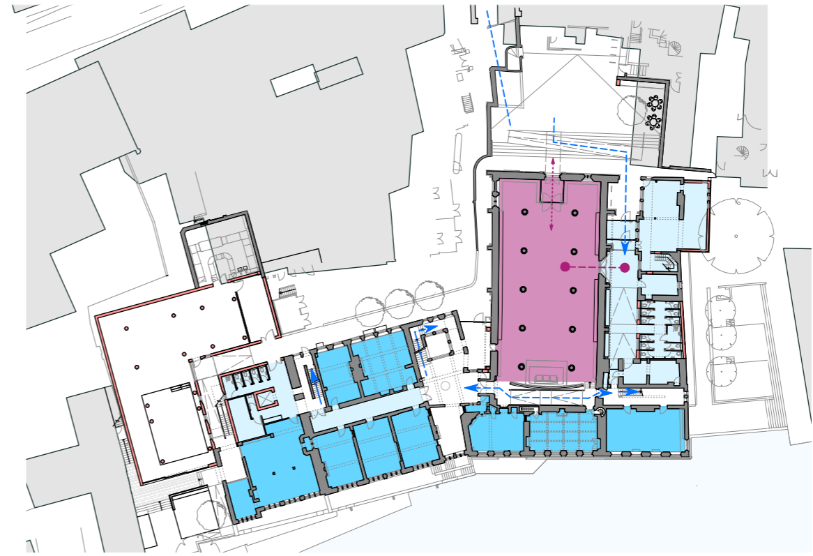
Diagram to show circulation and access for the office tenants, and Business Club at ground floor. Access is through the glazed South Range Slype space past the ancillary accommodation of café space, WC's and furniture store. Interconnectivity to the offices is provided behind the Guildhall screen via the proposed ramp.
